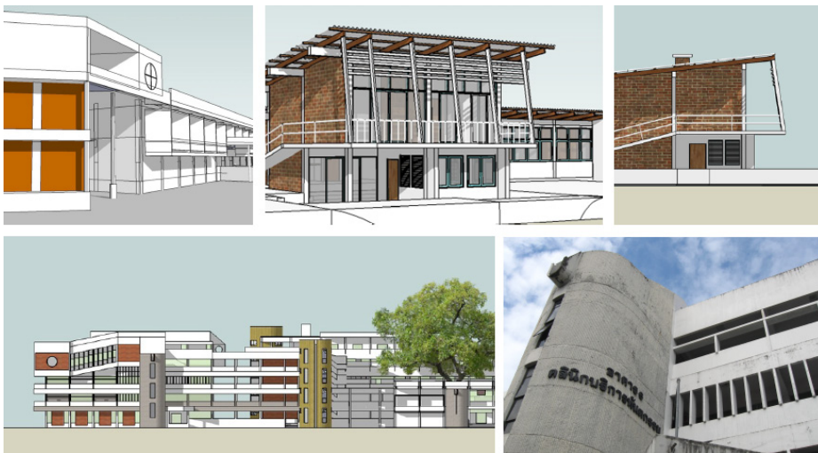
Figure 11. These images taken from various different buildings in Chiang Mai University to show how creative the designers were when they designed the concrete sun shading device, using as a second skin of the building, also allowing the building to have a good ventilation all day.
