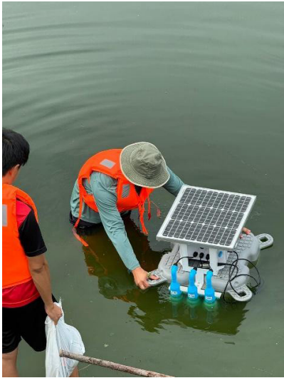
Figure 6. IoT water quality monitoring stations at Benjakitti wetland cell 1 inlet and outlet (top); close up of station configuration and water quality app (bottom)(photos by authors).
