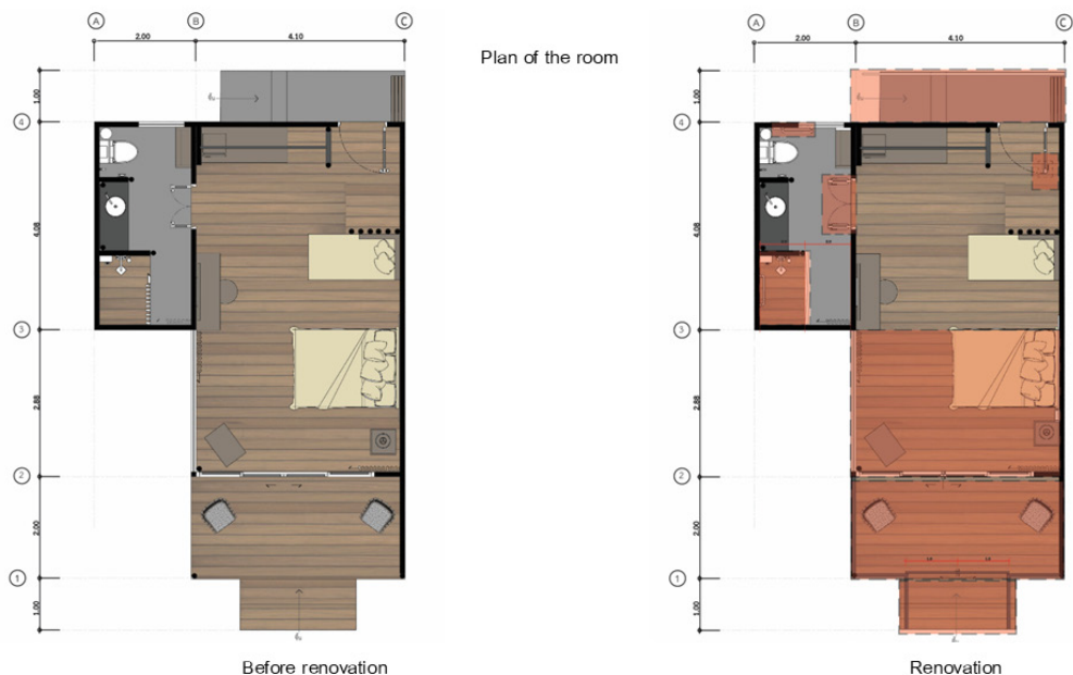
Figure 9. Plan of the room before renovation (left) and renovation proposed (right).
