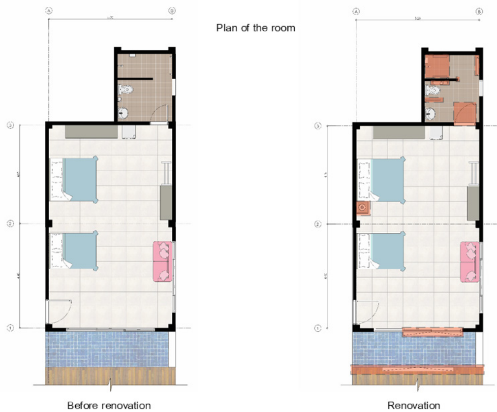
Figure 5. Plan of the room before renovation (left) and renovation proposed (right).
