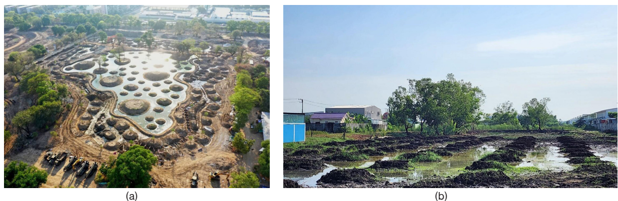
Figure 5. Comparison of construction techniques, (a) Benchakitti Forest Park's construction technique using the raised bed method; (b) a raised bed orchard in the central plain of the Chao Phraya River Basin.
