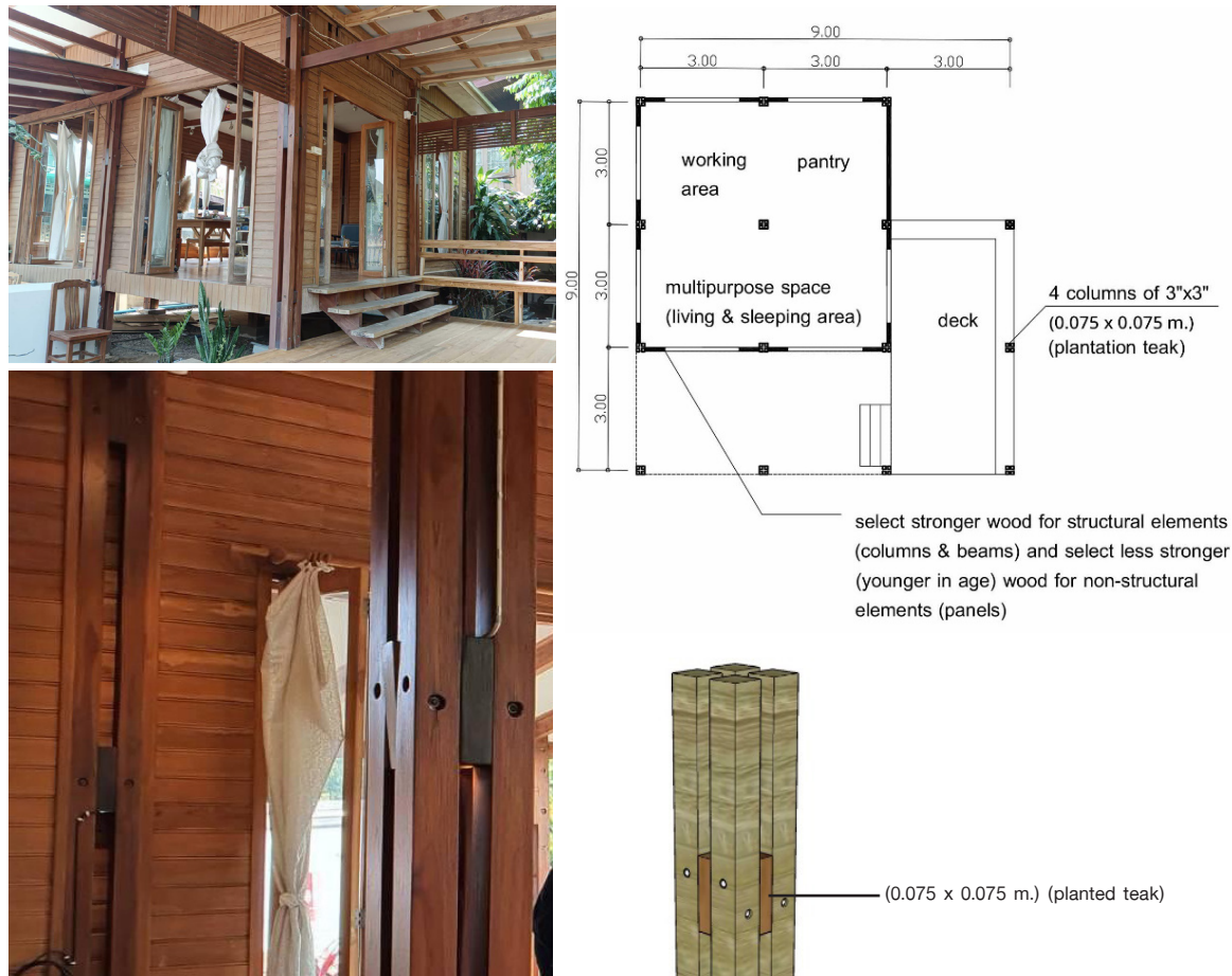
Figure 6. Planted teak knockdown house with smaller composite columns (Phrae case)
