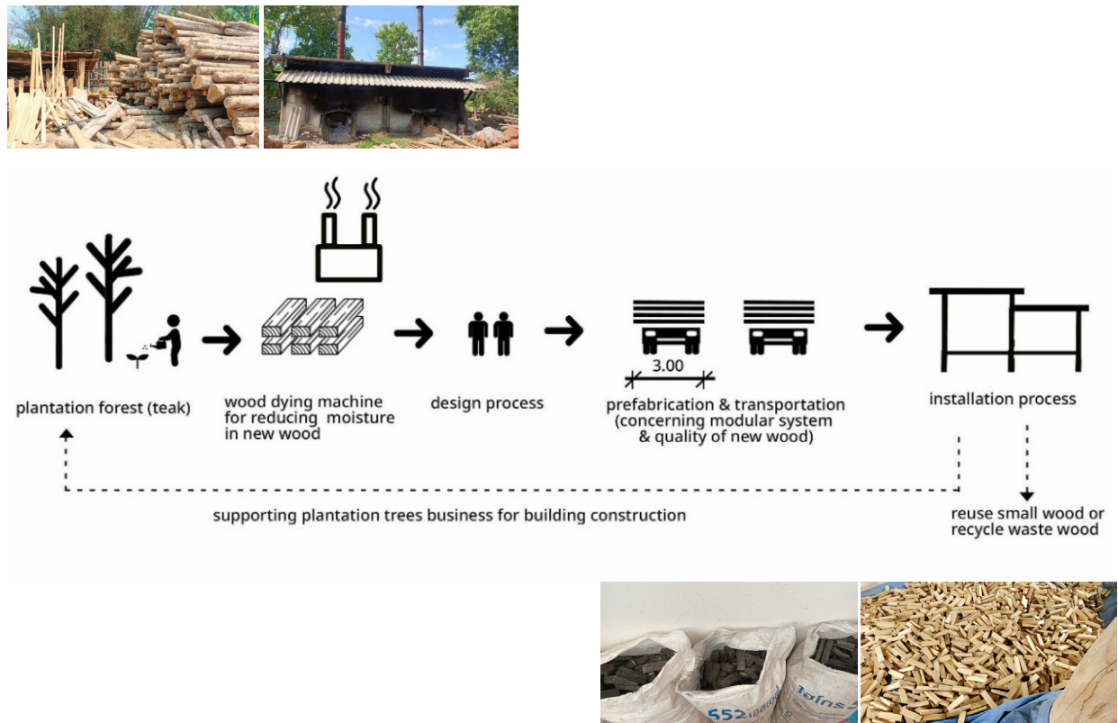
Figure 7. An overview of the construction process for knockdown wooden houses in category 3
