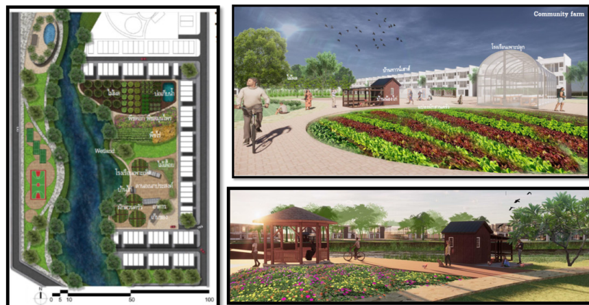
Figure 5 Enlarged plan view of Site 2.2, Agrihood design (left) showing the relative proximities of the main drainage canal, constructed wetlands, community gardens, and cluster homes. Perspective visions of the Agrihood design (top right and bottom right).
