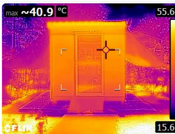
Figure 11. Temperature within the unit during noon time tested by thermal gun
