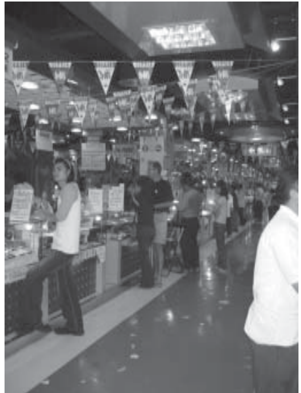
Figure 14 Dividing shopping malls into many small spaces adds more occupants per floor and makes the corridor narrower, which creates difficulty for evacuation in case of incidents that could occur.
