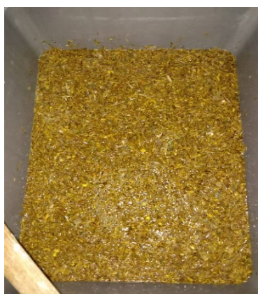
Figure 2: Immersion Process Using Sodium Hydroxide
