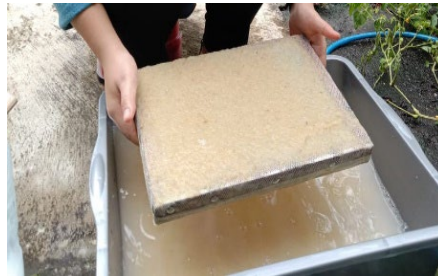
Figure 3: Pulp Filtering Process
