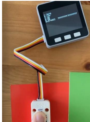
Figure 5: The Color Sensor Interpreting the HSL Value 8
