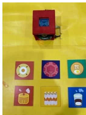
Figure 8: The IoT System Prototype that Pronounces the Name of Foods in Phuket Dialect when a Colored Card Is Placed on the Sensor
