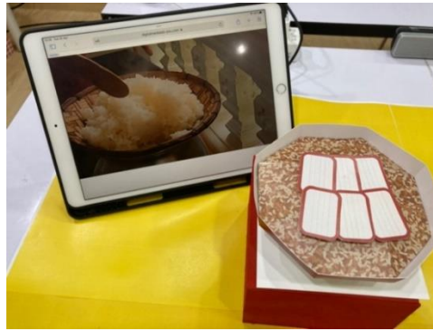
Figure 6: As Part of the Testing Process, a Paper Model of Ew Pueng Is Placed on the IoT Equipment (a Red Box) to Play the Cooking Process Video
