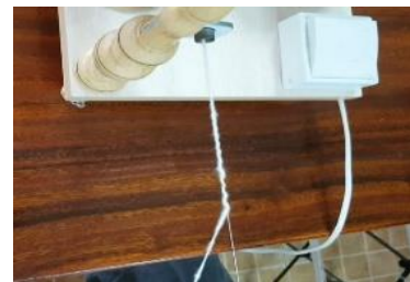
Step 3 Move yarns to about a 15-degree twist, respectively
