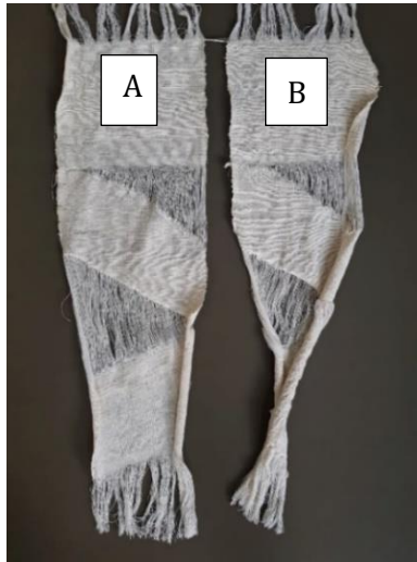
Figure 7: Experiment to Compare the Weft Yarn of Single Weft and Yarn Twist Weft
