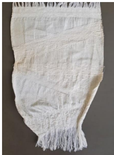
Figure 6: Experiment on Mixed Materials Twist and Various Weft Directions
