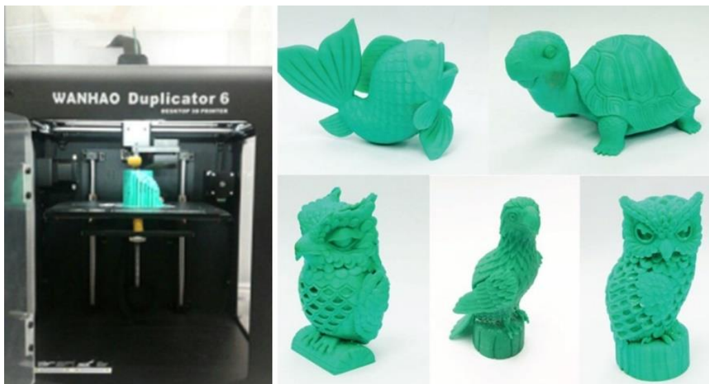
Figure 12-13: Miniature Prototype of Animal Sculpture, Dan Kwian Pottery by 3D Printer with PLA Filament
