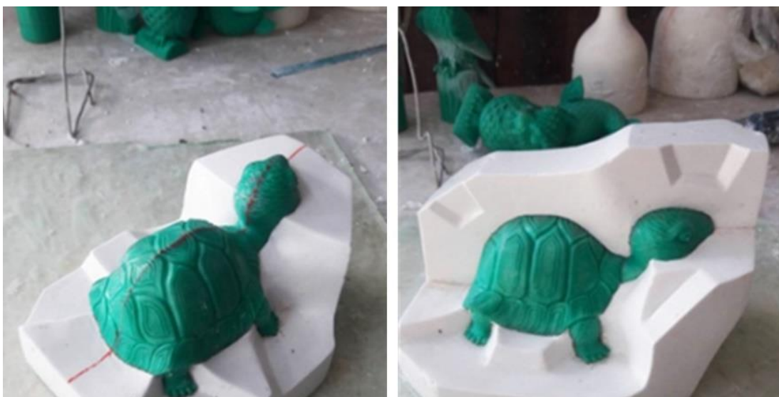
Figure 14-15: The Process of Making a Plaster Mold from a Miniature Prototype of a Clay Sculpture with a 3D Printer
