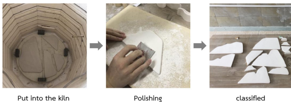
Figure 26 Biscuit firing and polishing process
