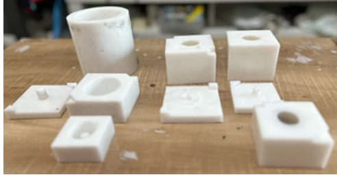
Figure 9 Silicone Mold Creation
