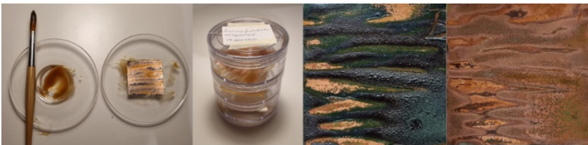
Image 2 – The procedure of applying Tamarind Paste solution to copper sheet and the patina result
