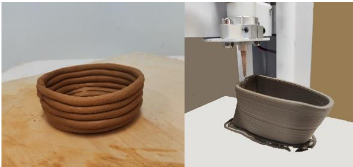
Figure 2 Ceramics made with panning clay strips and 3D printing Source: From the author
