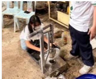
Figure 6. Press molding of plant pots
