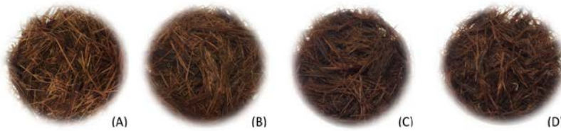
Figure 3. Pulp of nipa stalk after soaking in NaOH at different concentration, (A) 0.5%, (B) 2%, (C) 5% and (D) 10%
