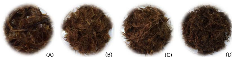
Figure 2. Pulp of nipa leave after soaking in NaOH at different concentration, (A) 0.5%, (B) 2%, (C) 5% and (D) 10%
