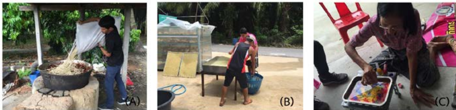
Figure 8. Knowledge transfer nipa paper production technology from this research to Palian river basin community, (A) preparation of nipa wastes, (B) nipa casting and (C) color dyeing of nipa paper
