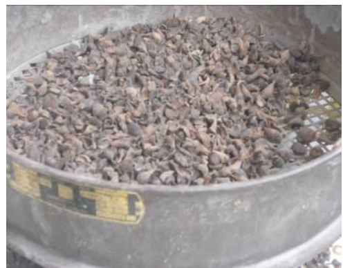
Figure 2 Oil palm shell retains on sieve No. 3/8
