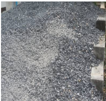
Figure 1 Coarse aggregate size of 3/8 inch
