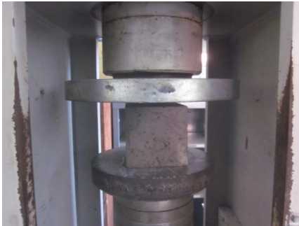
Figure 3 Compressive strength testing
