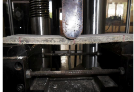
Figure 4 Flexural strength testing
