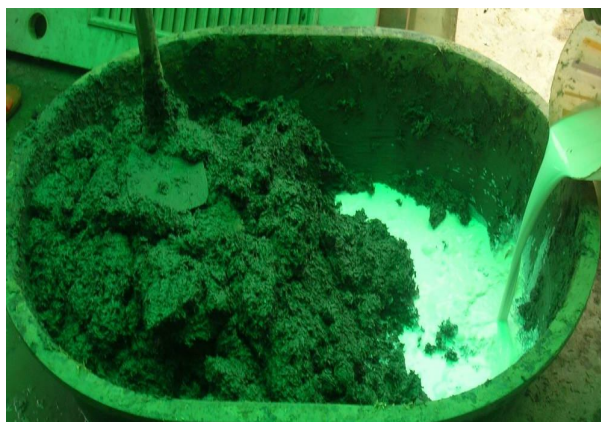
Figure 4 The mixing of natural latex and clay
