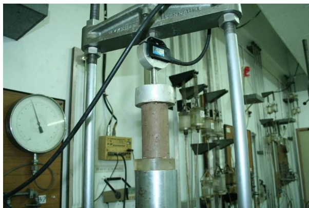
Figure 5 The unconfined compression test of compacted clay liners
