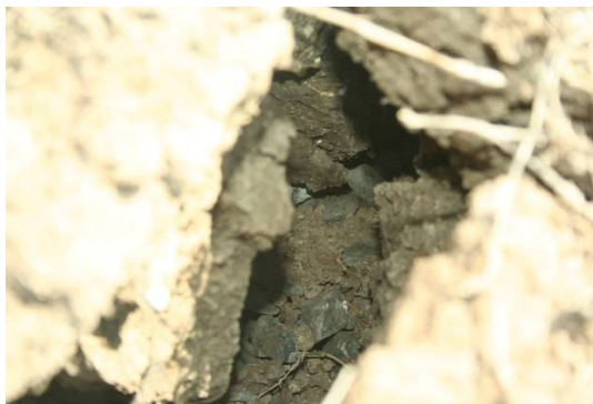
Figure 1 The big cracking of compacted clay liner (top soil) of landfill
