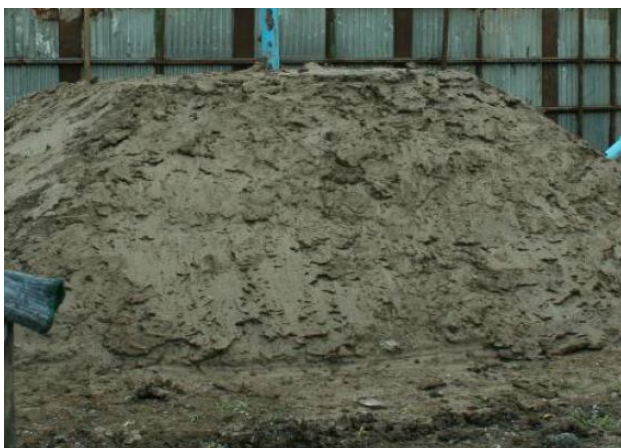
Figure 6 The compacted clay liner (top soil) of landfill which was mixed with natural latex
