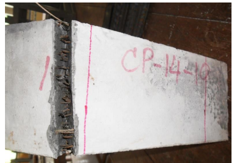
Figure 6 Failure of sample under the flexural strength
