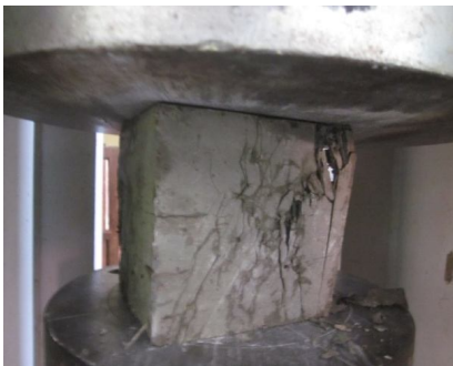
Figure 5 Failure of sample under the compressive strength
