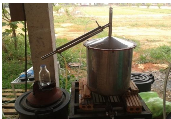
Figure 2 Wood vinegar distillation system and (A) wood vinegar distilled (B) crude wood vinegar
