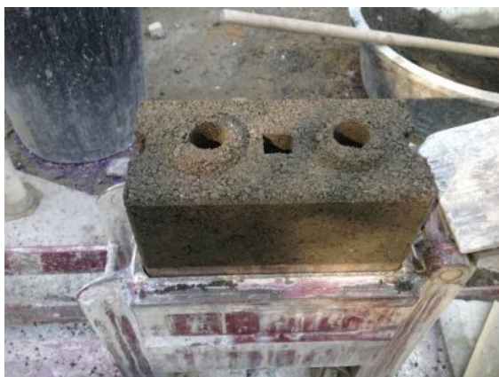
Figure 4 Interlocking block after molding
