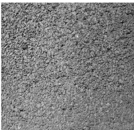
Figure 5 Surface of volcanic rock waste paving block
