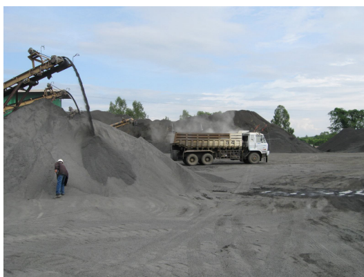
Figure 2 Volcanic rock waste in basalt mine from Buri Ram province
