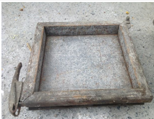
Figure 4 Mold of paving block
