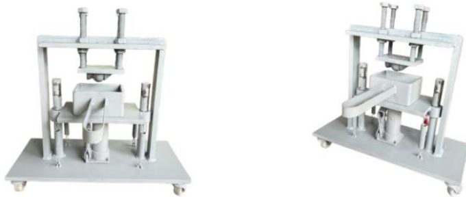
Figure 7. Completed rice straw cushioning material product extruder
