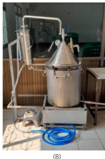
Figure 2. Citronella oil distillation equipment: (A) Construction process, (B) Completed
