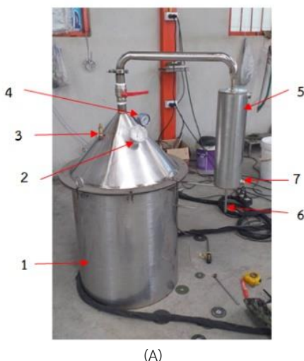
Figure 2. Citronella oil distillation equipment: (A) Construction process, (B) Completed
