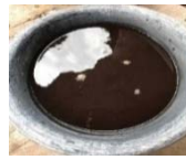
Figure 3. The process of extracting color by heat in a ratio of 1 kg of teak per 1 liter of lye
