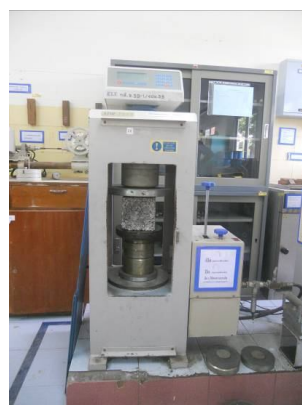
Figure 4 Compressive strength testing
