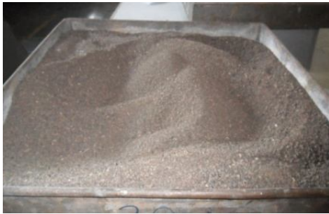
4A) Palm shells passing sieve number 8
