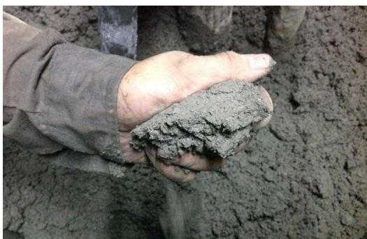
Figure 8 Suitable moisture test of concrete block mixture
