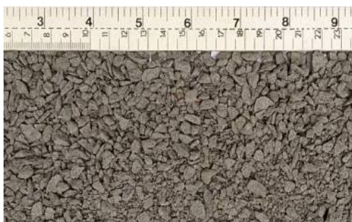
Figure 5 Quarry waste from volcanic rock quarry (crushing machine no.2) (for VC2 concrete block)
