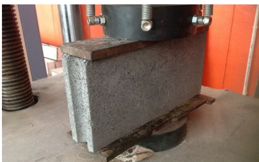
Figure 10 Compression test of concrete block
