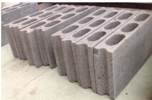
Figure 9 Concrete blocks using volcanic rock waste
