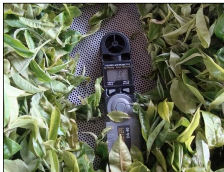
Figure 7 Anemometer on the withered tea air stove
