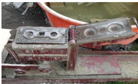
Figure 3 Manual compression molding machine
