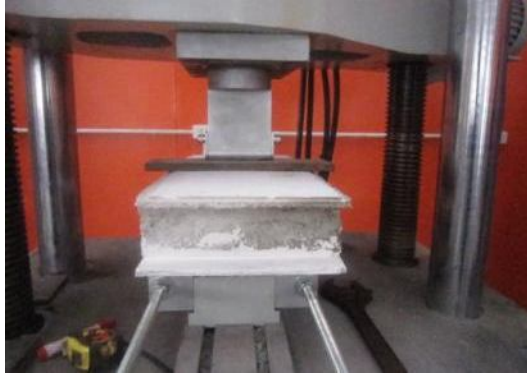
Figure 6 Transverse bending strength test of volcanic rock waste paving block
