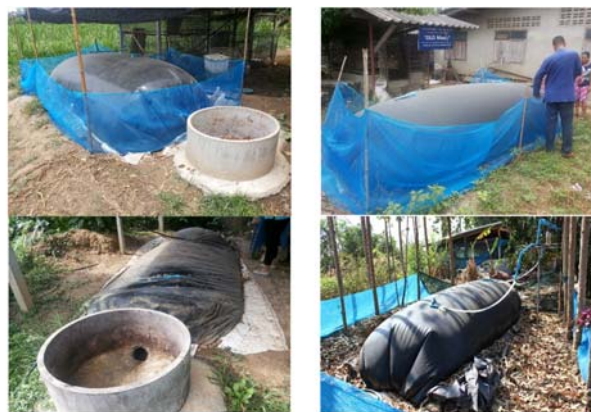
Figure 4 Biogas production process using bio extract in plastic bag in the studied area
