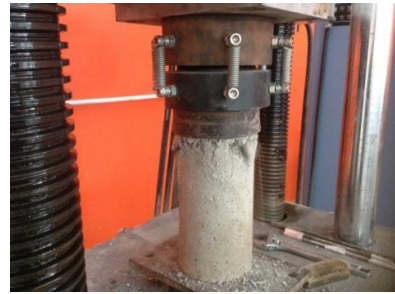
Figure 3 The compressive strength test of concrete cylinder mixed with oil-palm waste ash and crushed dust
