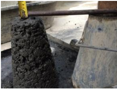
Figure 2 The slump test of flesh concrete mixed with oil-palm waste ash and crushed dust
