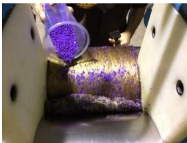
Figure 4 Blending of admixture in two-roll mill machine
