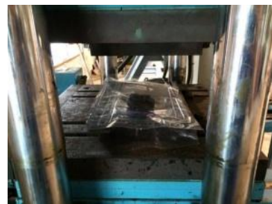
Figure 5 Putting the blended admixture into rubber compression machine
