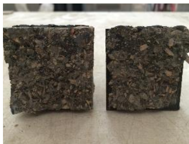
Figure 6 Cracking texture of particle board wall mixed with cement and cassava pit waste after the tensile strength test
