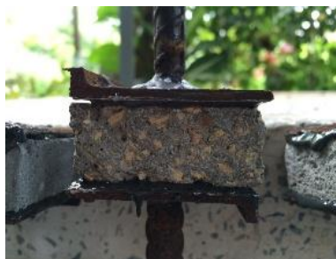
Figure 5 Particle board wall mixed with cement and cassava pit waste sample for tensile strength test
