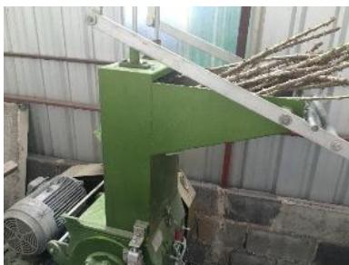
Figure 1 Grinding of cassava pit waste with the plastic granulator and sieve no.4
