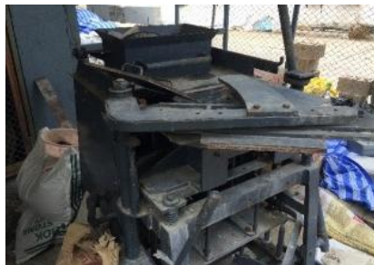
Figure 3 Particle board wall compression with shaking type compressor
