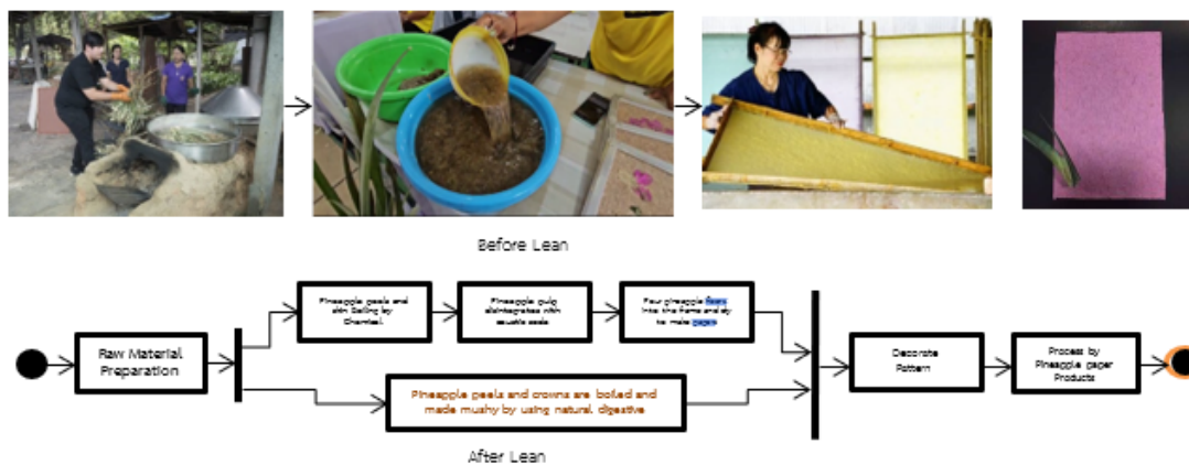
Figure 4 Pineapple paper process Flowchart.
