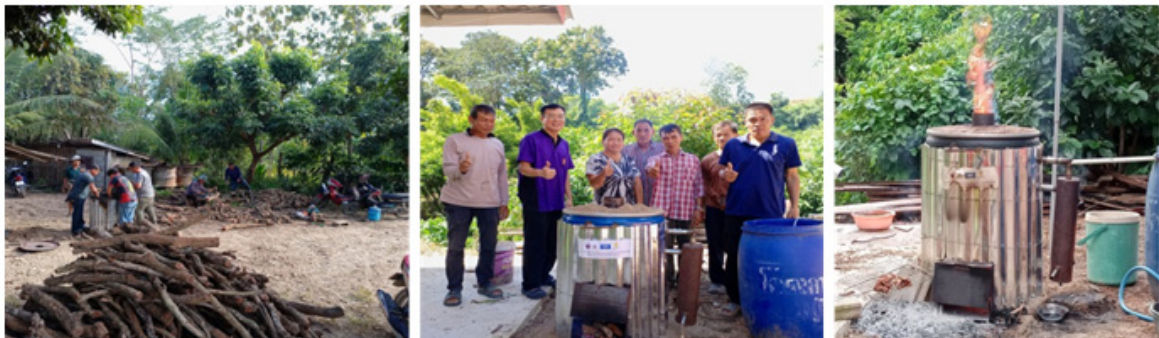
Figure 7 Management of waste agricultural by-products (longan branches) by burning them in a low-pollution wood vinegar and charcoal kiln.
